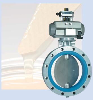
Tight shut-off Butterfly Valve in lug type execution for installation between flanges according to DIN 2501 and ANSI Class 150 with centric disc.
