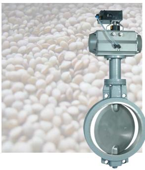
Shut-off Butterfly-/ Regulating Valve in wafer type design for installation between flanges according to DIN 2501 and ANSI Class 150, metallic seal, with centric disc.
