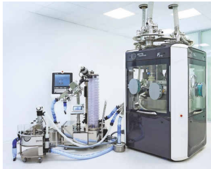
Example of a total solution meeting Containment Guard 3: FE75 tablet press with containment package and process equipment
