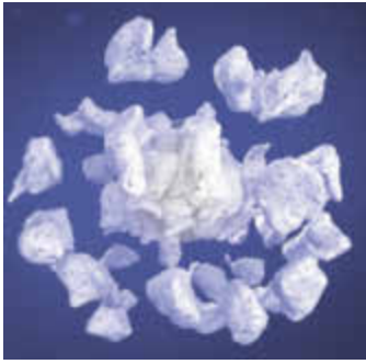
Very large agglomerates only break up after passing through a second time
