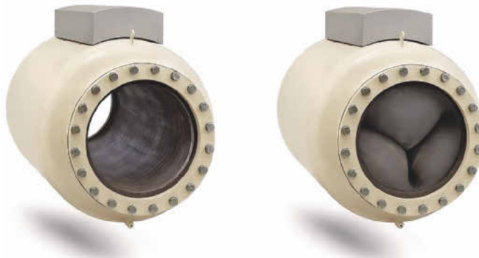
Quench valves, open and closed: these valves are activated in response to a rise in pressure or the formation of flames
